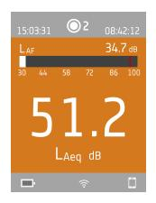
Press ▲ and ▼ briefly to scroll through measurement displays. Press ◀ and ► briefly to scroll through the parameters for each display.
