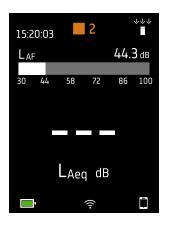
The number in the centre is the measurement number. The first measurement of every day is number 1. The number increments with each new measurement.
