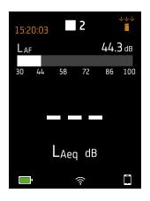
When idle, the instrument displays the current time (to the left) and input settings (to the right).
